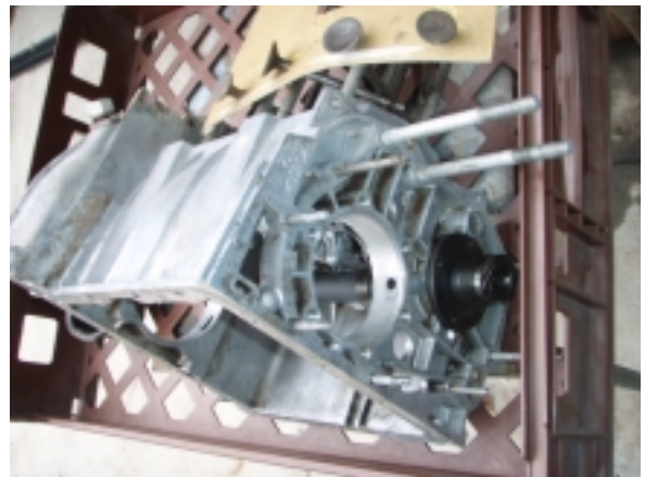
Crankcase ready for measuring
